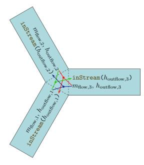
**Figure C.2:** Exemplary connection set with three connected components.
