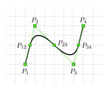
**Figure 18.1:** Line with smooth = Bezier. The four line points  $P_1, \ldots, P_4$  result in two quadratic splines and two straight line segments.
