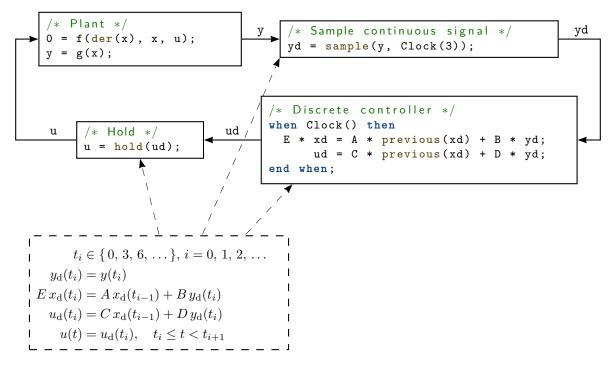
**Figure 16.1:** A continuous plant and a sampled data controller connected together with sample and (zero-order) hold elements.
