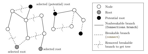
Figure 9.2: Example of a virtual connection graph.
