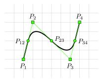
**Figure 18.1:** Line with **smooth = Bezier**. The four line points  $P_1, \ldots, P_4$  result in two quadratic splines and two straight line segments.
