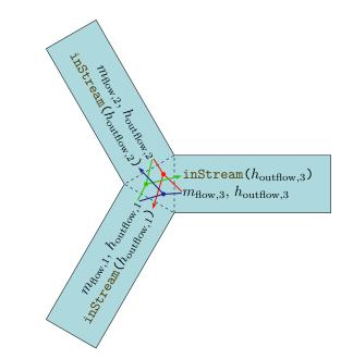
Figure C.2: Exemplary connection set with three connected components.
