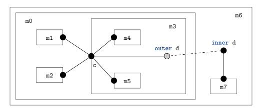
Figure 9.1: Example for inside and outside connectors.
