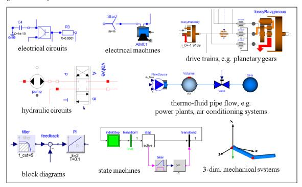
A schematic consists of connected components, like a resistor, or a hydraulic cylinder. A component has connectors (often also called ports) that describe the interaction possibilities, e.g., an electrical pin, a mechanical flange, or an input signal. By drawing connection lines between connectors a physical system or block diagram model is constructed. Internally a component is defined by another schematic, or on "bottom" level, by an equation-based description of the model in Modelica syntax.
