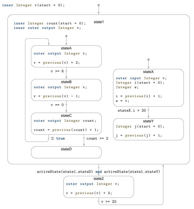
Figure 17.2: Example of a hierarchical state machine.
