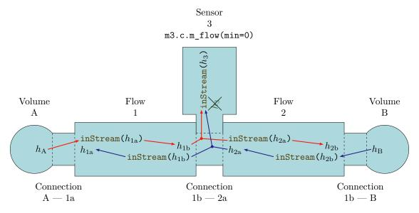
Figure C.3: Example series connection of multiple models with stream connectors.
