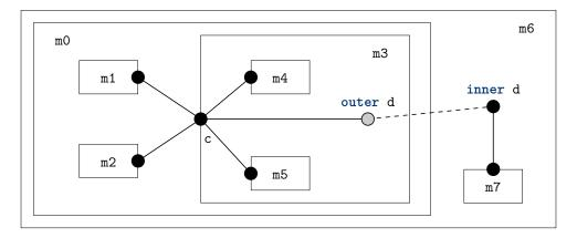
**Figure 9.1:** Example for inside and outside connectors.
